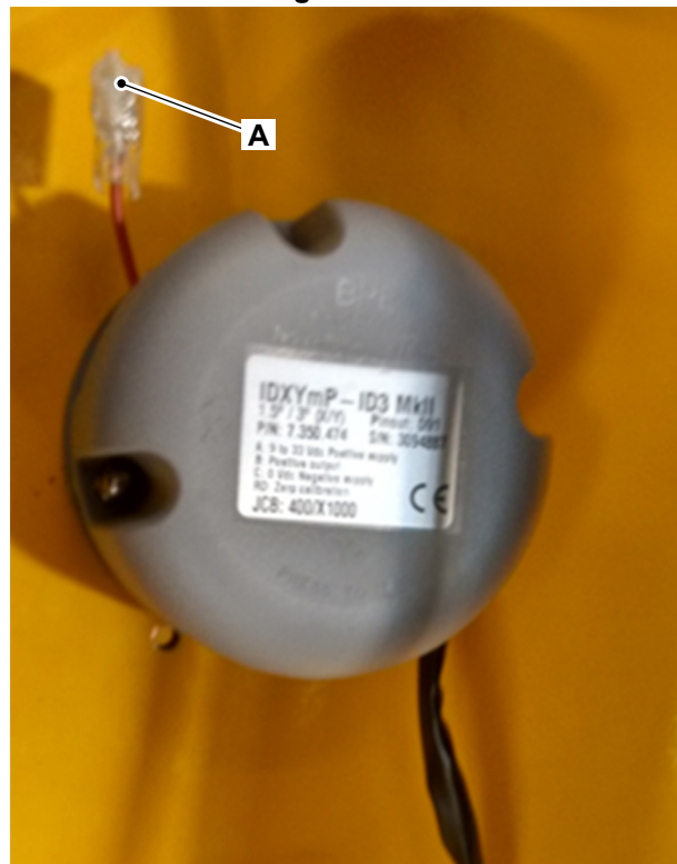
A Electrical terminal
