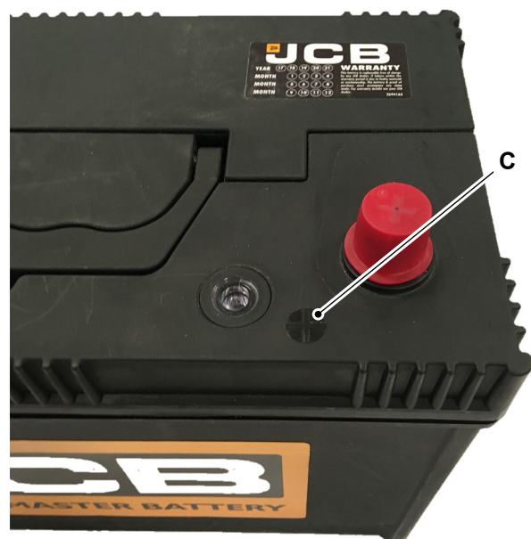
C Positive battery-terminal identification
