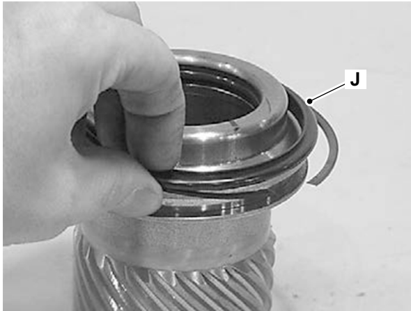
J Outside diameter piston seal
