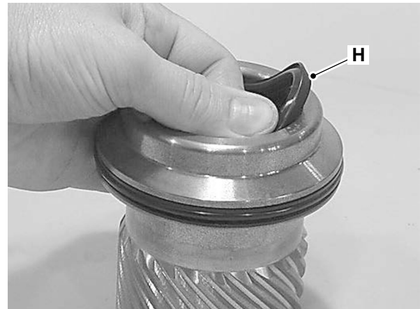
H Inside diameter piston seal (T-seal)
