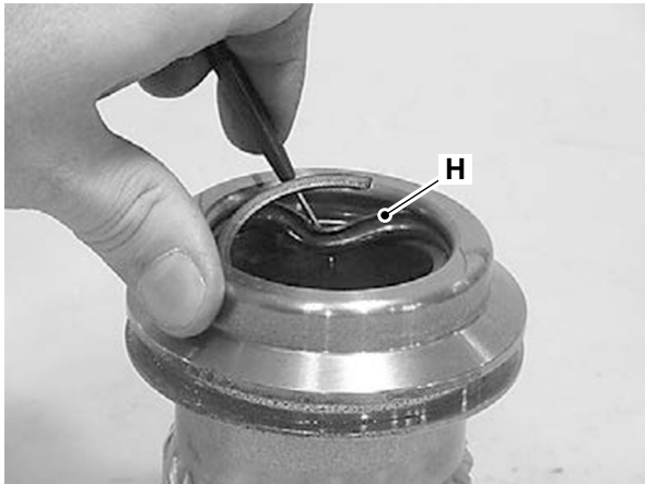
H Inside diameter piston seal
