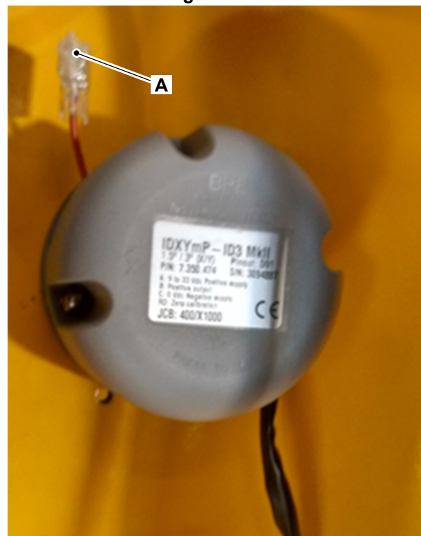
A Electrical terminal
