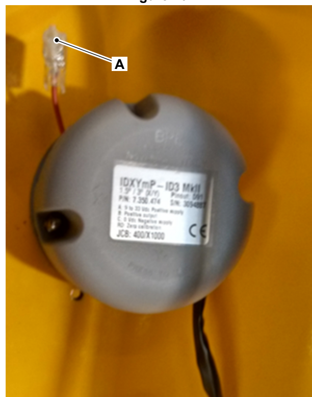
A Spare cable
