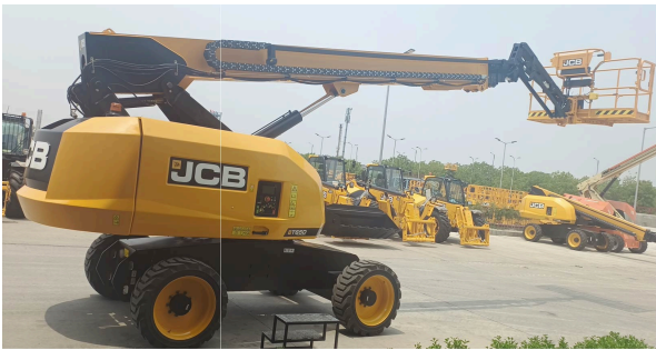
Figure 185. Boom Lift Upwards at 10° angle
