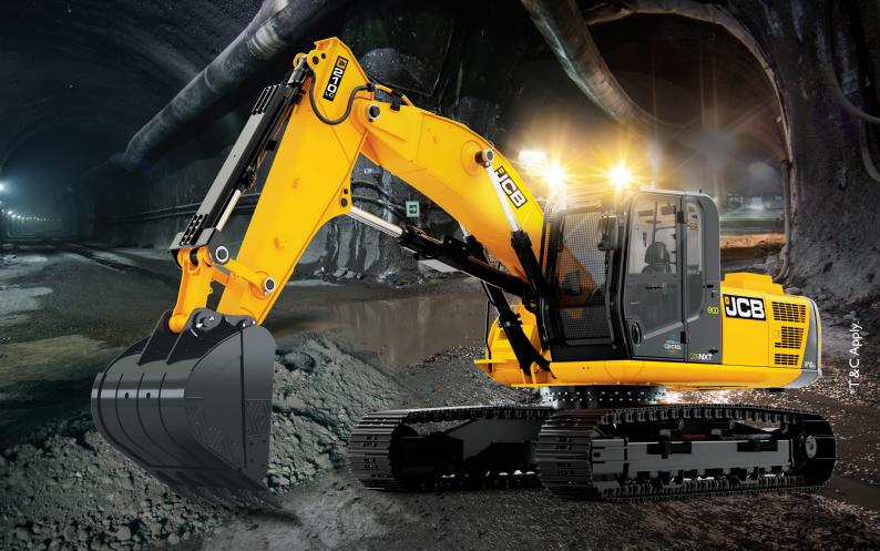
Engine Power: 104 kW (140 hp) | Bucket Capacity: 0.9 cu.m GP / 0.9 cu.m(HD) Operating Weight: 21,250 kg (LC)
