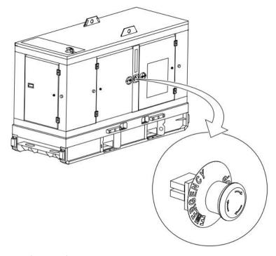
NOTE: Activation of either of the emergency stop buttons will put the generator into a fault mode.
