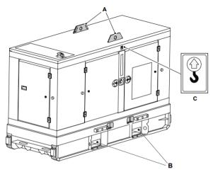
For movement on site the optional fork pockets enable the generating set to be lifted and shifted by forklift or telescopic handler. The fork pockets are sized and spaced to allow lifting by equipment with a standard fork carriage.
