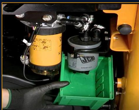
Drain fuel sedimentary. Do not disconnect the water in fuel connector.
