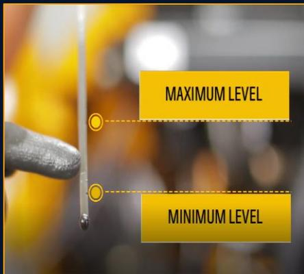
**Check the Engine oil level**
