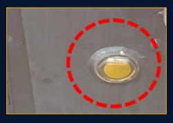
Hydraulic Oil level to be visible in gauge.
