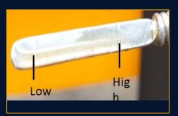
Check engine oil level (To be between high and low mark).
