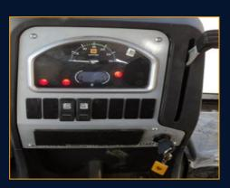
Start machine for I5-20mins in idle. Operate all gears, steering, brakes, services and stroke all rams in hot condition.
