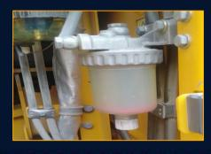
Check for leakages and drain fuel filter, water separator and FIP.
