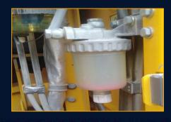
Check for leakages and drain fuel filter, water separator and FIP.
