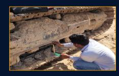
Lubricate tracks, linkages and joints (adjust track tension)
